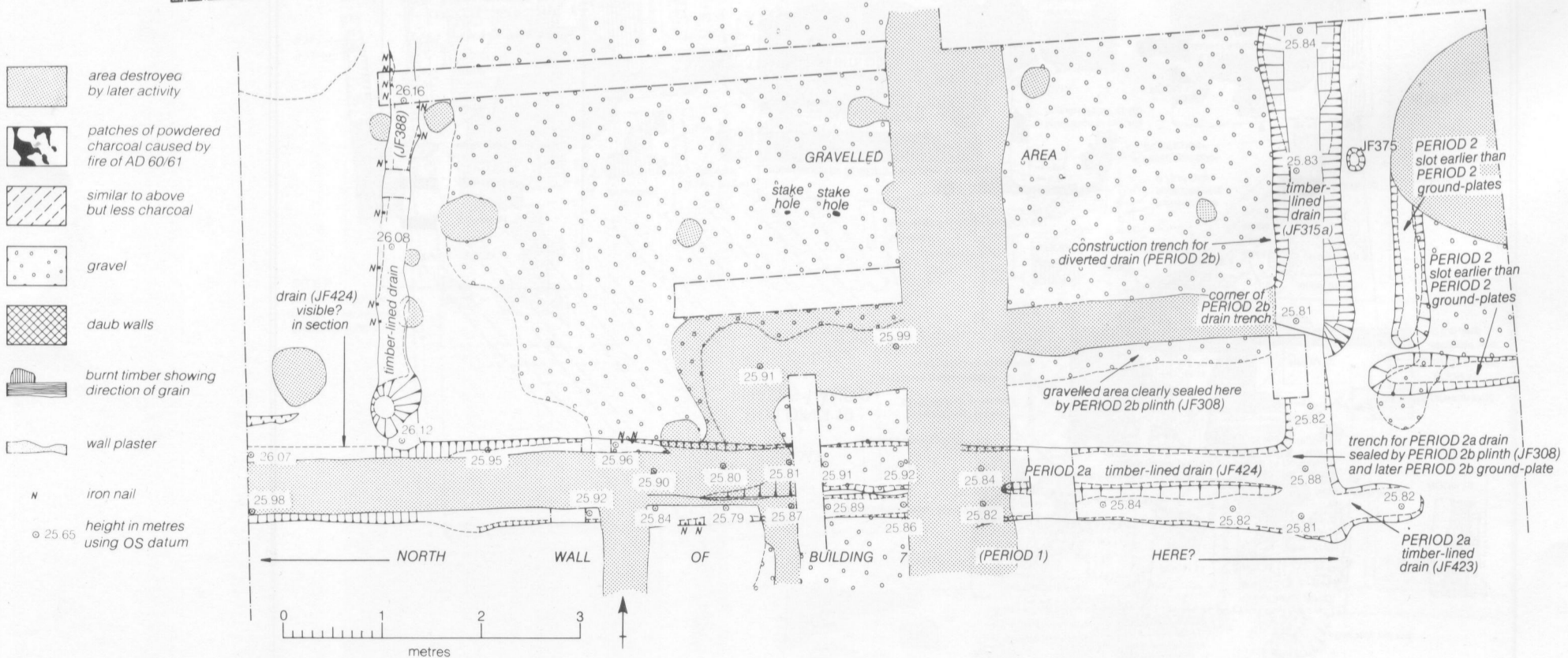
Fig 29 The southern end of Building 8 with first phase of drainage system shown separately below. 1:60. [Pages 40-2]
