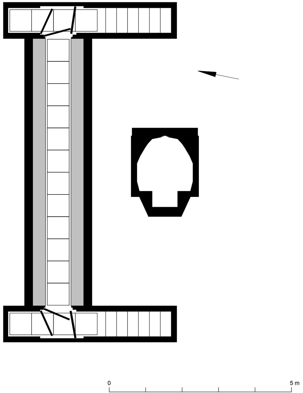
Fig 15 Development Area 8: air-raid shelter WBF102 - plan and cross-section.
