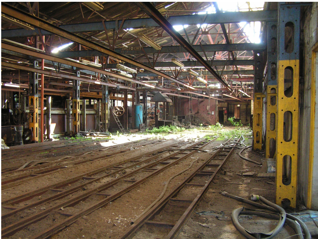
A1.18 Main foundry casting floor with overhead monorail metal-handling system, view south-east.
