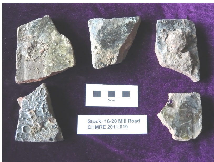
Plate 2: peg-tiles with bubbled green glaze and adhering pot fragments
