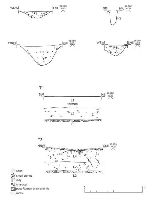
Fig 3 Feature sections (F1-4) and representative trench sections (T1-2).
