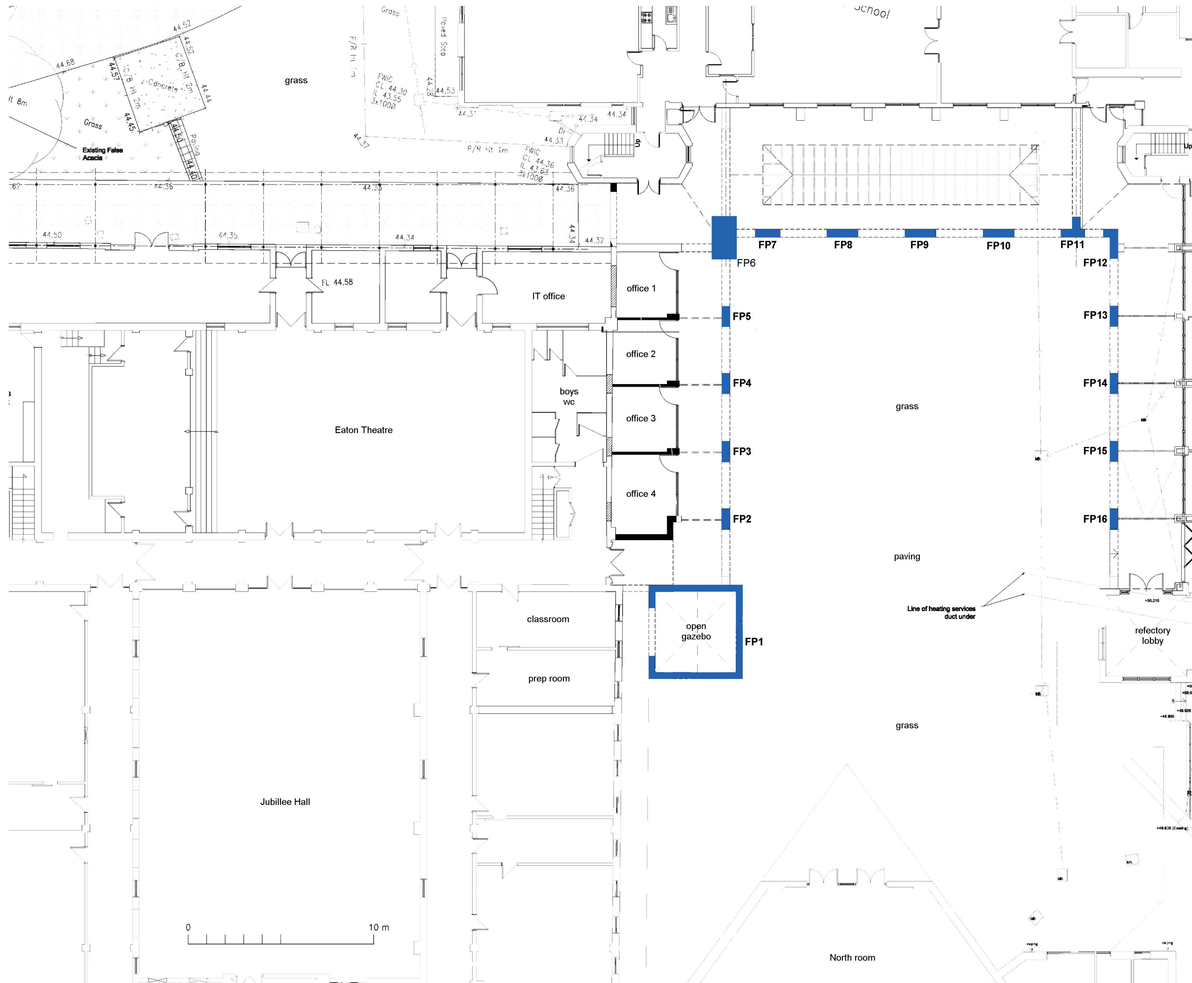
Fig 2 Foundation pads (in blue).
