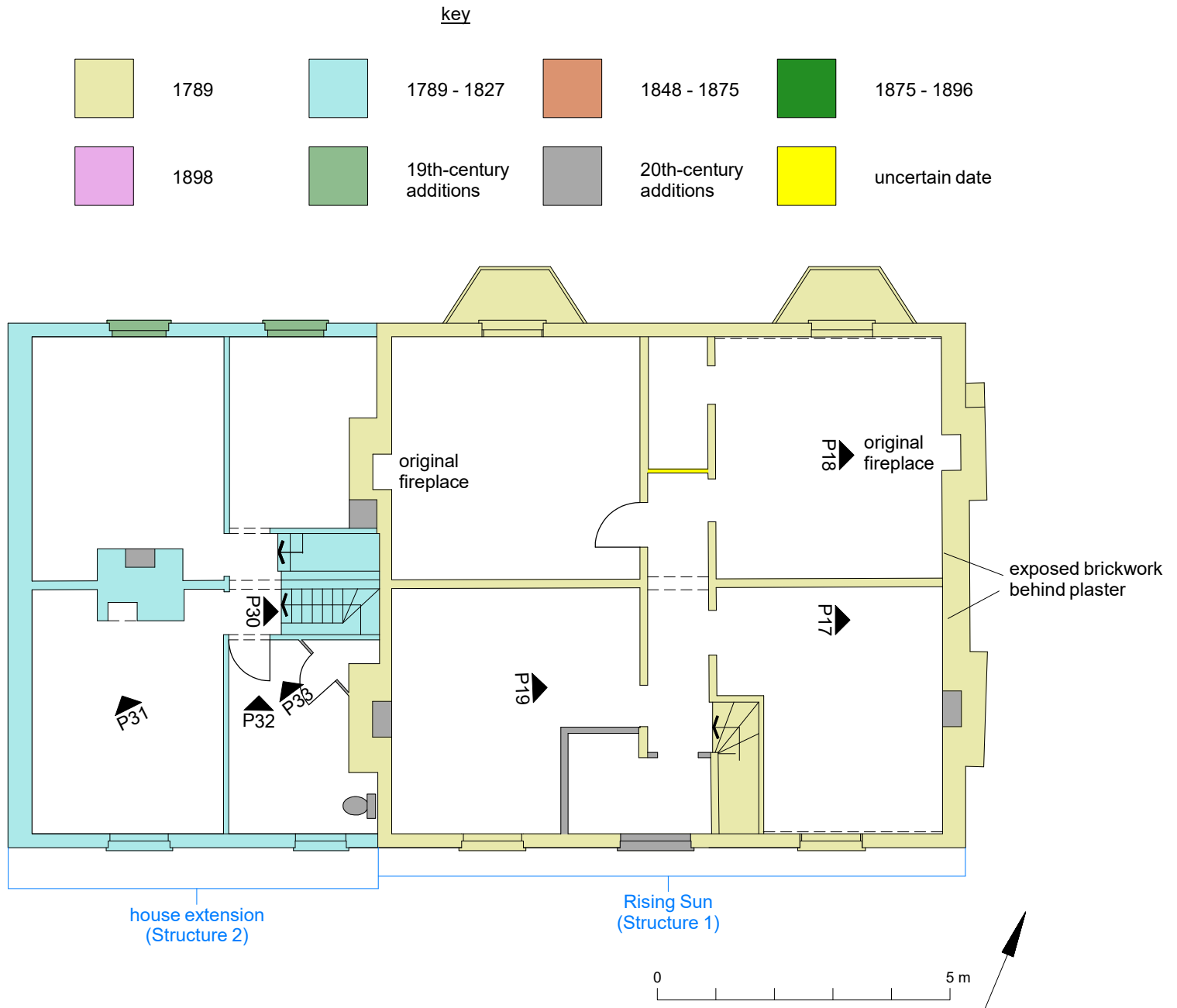
Fig 5 First-floor plan of Structures 1 and 2. Location and direction of photographs reproduced in text shown, along with phasing.
