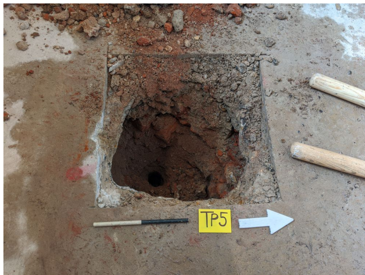
Photograph 1 Test-pit 5 fully excavated
