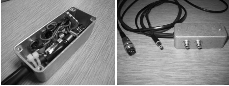
(a) The 9 Volt DC-to-DC box with its internal components visible (b) The 9 Volt DC-to-DC box and connectors
