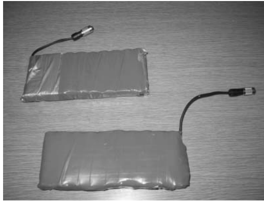
Figure 4.9: The two battery packs assembled and wrapped in insulating tape
